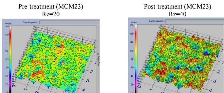
Fig. 6. Rz values and topographic maps from different fragments of wall-paintings from Mitreo’s House comparing pre- and post-treatment with Estel 1000<sup>®</sup> on IGEO case
