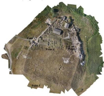
Fig. 12. Locations of the 5 Ground Control Points (GCP)
