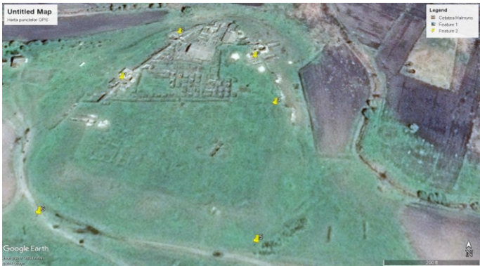
Fig. 3. Control points determined before the actual flight
