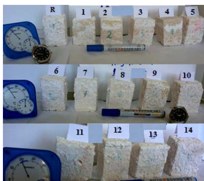
Fig. 6. Photo-documentation for the control R and fourteen limestone samples, treated with the resins under investigation, after 10 cycles of artificial weathering with anhydrous \text{Na}_2\text{SO}_4
