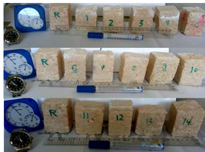
Fig. 5. Photo-documentation for the control "R" and fourteen limestone samples, treated with the resins under investigation, after 6 cycles of artificial weathering with anhydrous Na 2 SO 4
