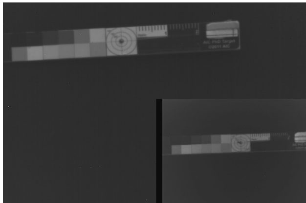
Fig. 5. The AIC Photo Documentation Target [11] seen by the Xenics Bobcat 640 (640x512pixels) and the Indigo System Merlin InGaAs camera (320x256pixels), in the insert, bottom right. The images are at their actual ratio. The cameras were at the same distance (2,2m) and had the same 200mm lens mounted
