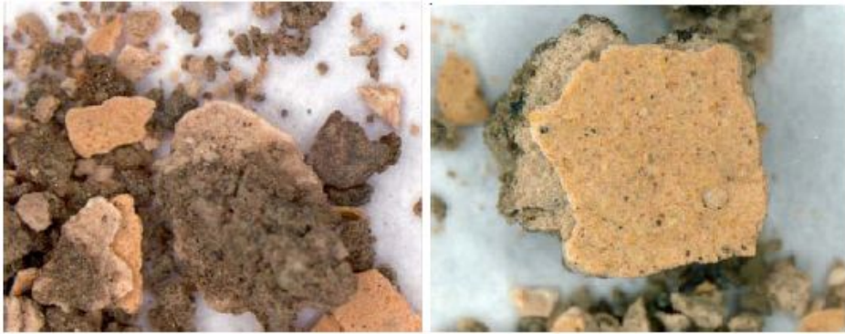
Fig. 8. Stereomicroscopic image of painted mortar of cave no. 15, Ajanta
