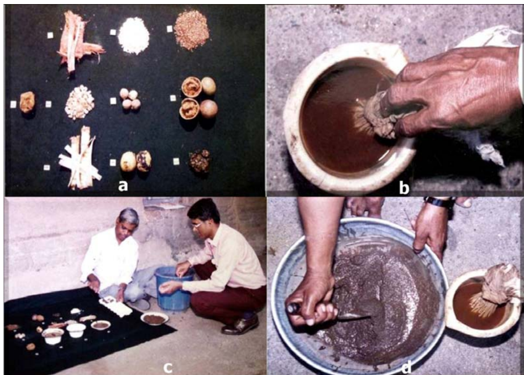
Fig. 3. Shows various steps in the preparation of mud mortar as per ancient recipe: a - ingredients for the preparation of mud mortar, b - preparation of adhesive extract, c - preparation of soil + lime + aggregates mixture, d - final step showing the preparation of mud mortar)
