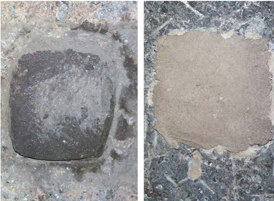
Fig. 4. Application of mud mortar on basaltic stone
